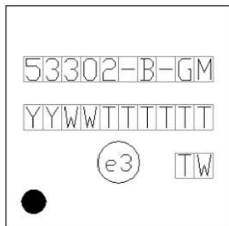
Figure 8.4. Si53302 Top Marking
