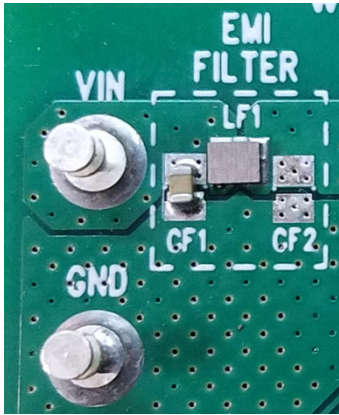
Figure 5. LC Filter on VIN Line
