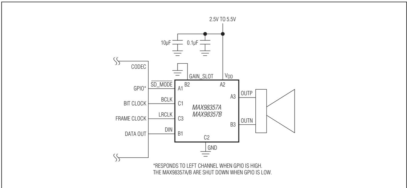
Figure 16. Left-Channel PCM Operation with 12dB Gain
