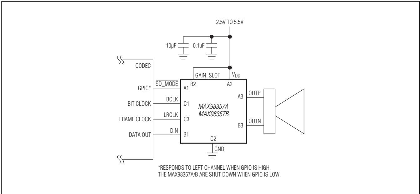
Figure 15. Left-Channel PCM Operation with 6dB Gain
