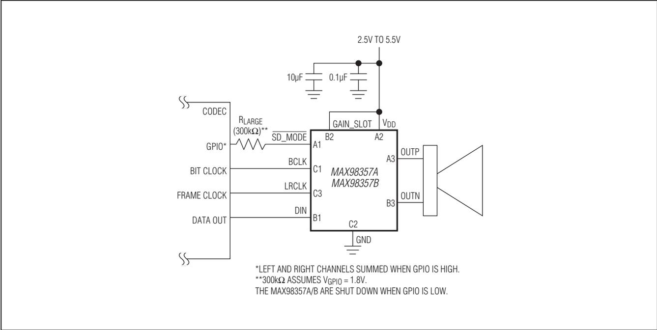
Figure 18. (Left/2 + Right/2) PCM Operation with 6dB Gain
