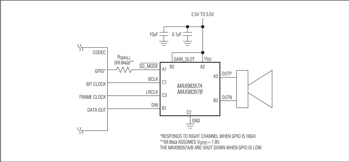
Figure 17. Right-Channel PCM Operation with 6dB Gain
