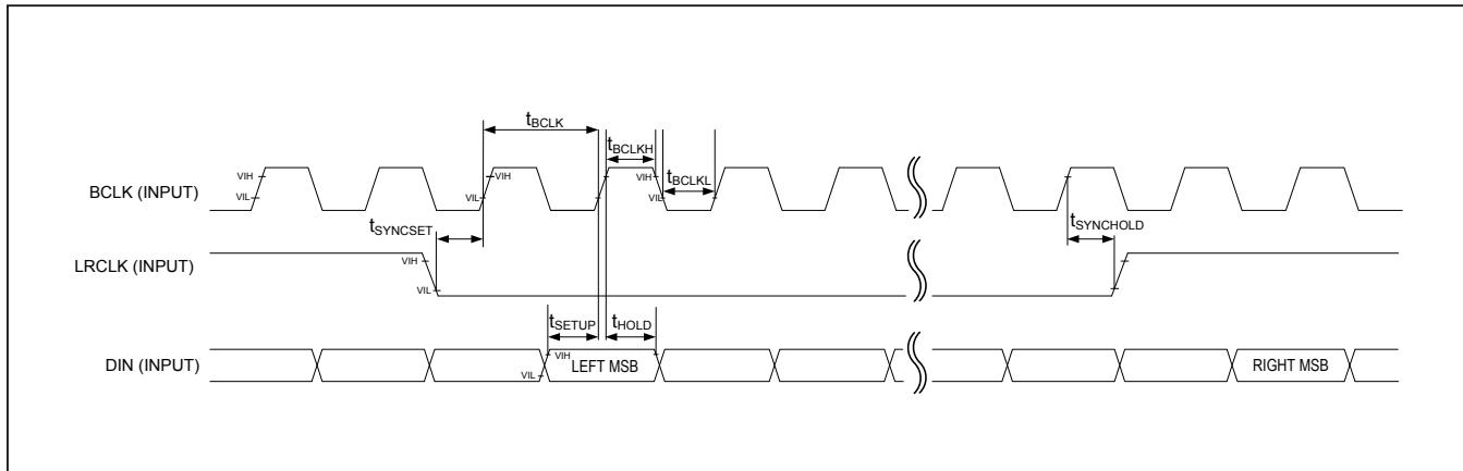
Figure 1. I<sup>2</sup>S Audio Interface Timing Diagram (MAX98357A)
