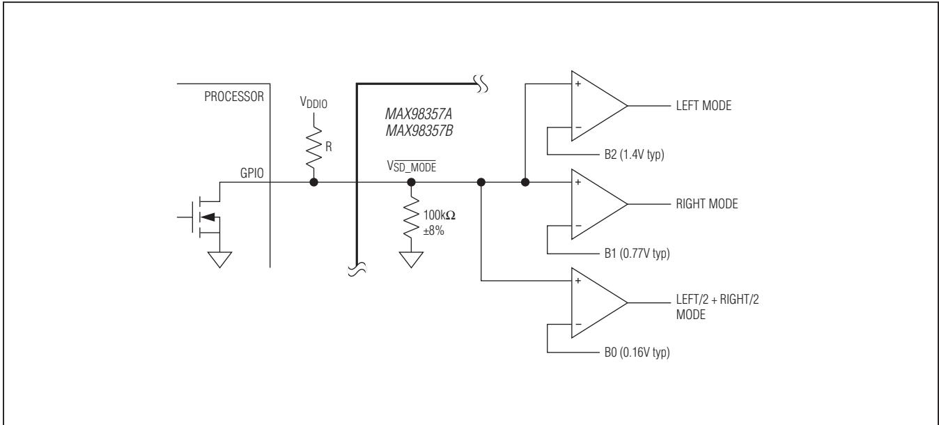
Figure 4. SD\_MODE Resistor Connected Using Open-Drain Driver
