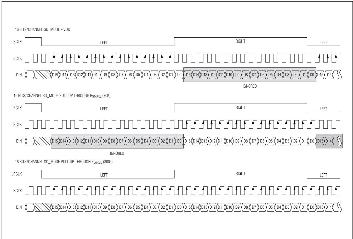
Figure 6. MAX98357A I<sup>2</sup>S Digital Audio Interface Timing, 16-Bit Resolution
