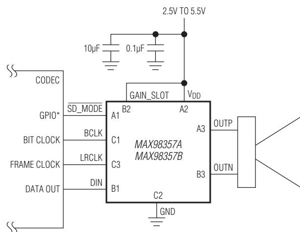
Figure 15. Left-Channel PCM Operation with 6dB Gain
