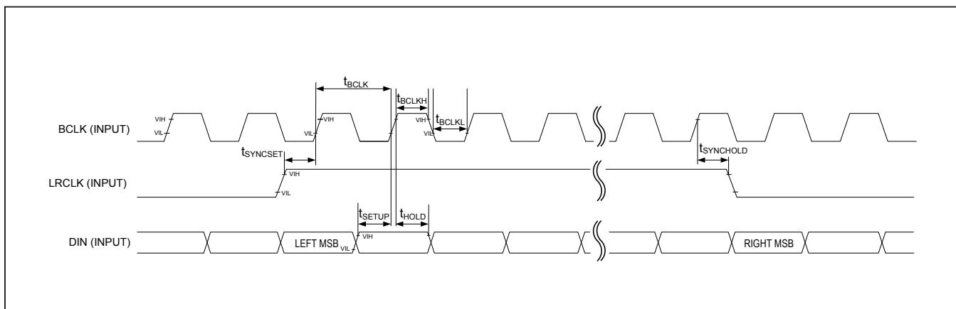
Figure 2. Left-Justified Audio Interface Timing Diagram (MAX98357B)
