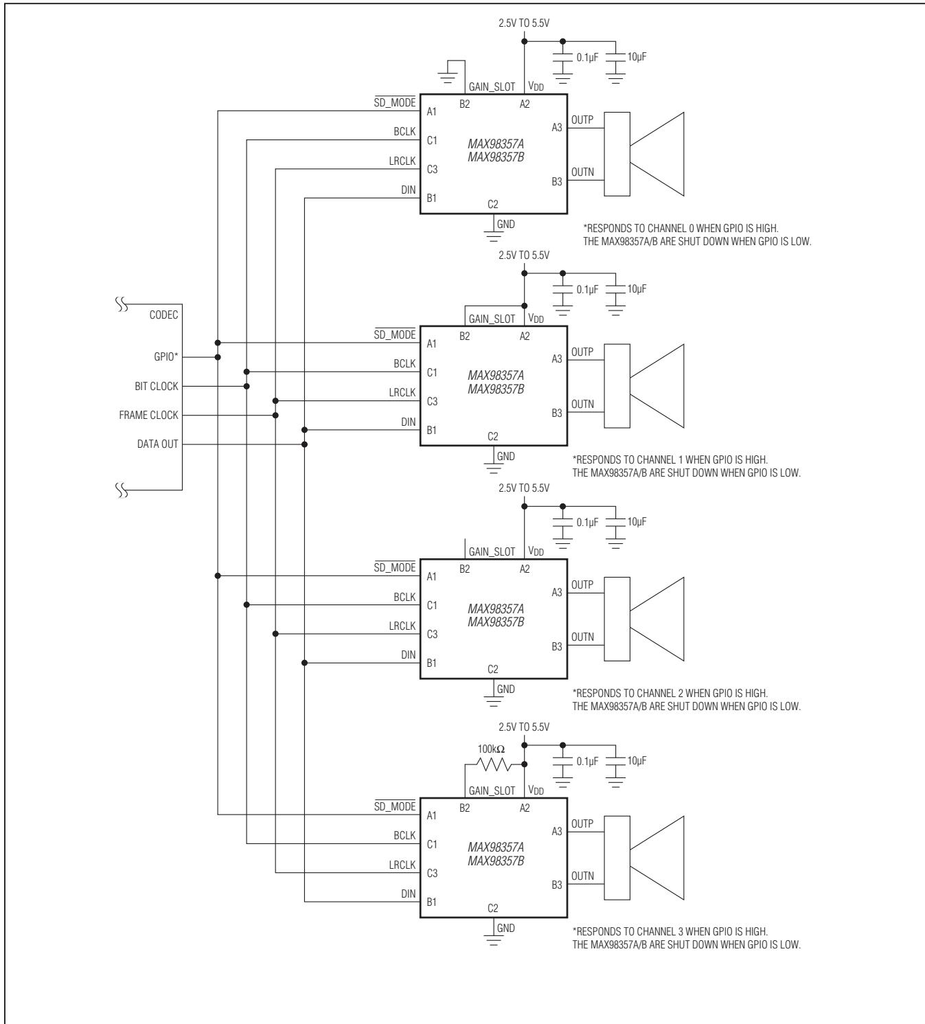
Figure 20. Channel TDM Operation (Gain Fixed at 12dB)
