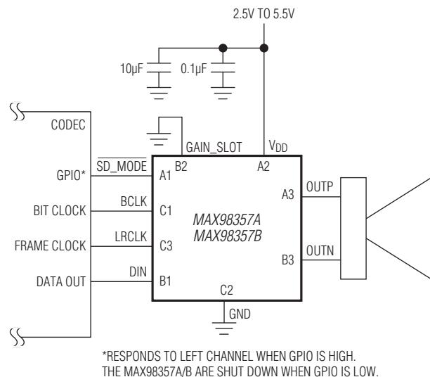
Figure 16. Left-Channel PCM Operation with 12dB Gain
