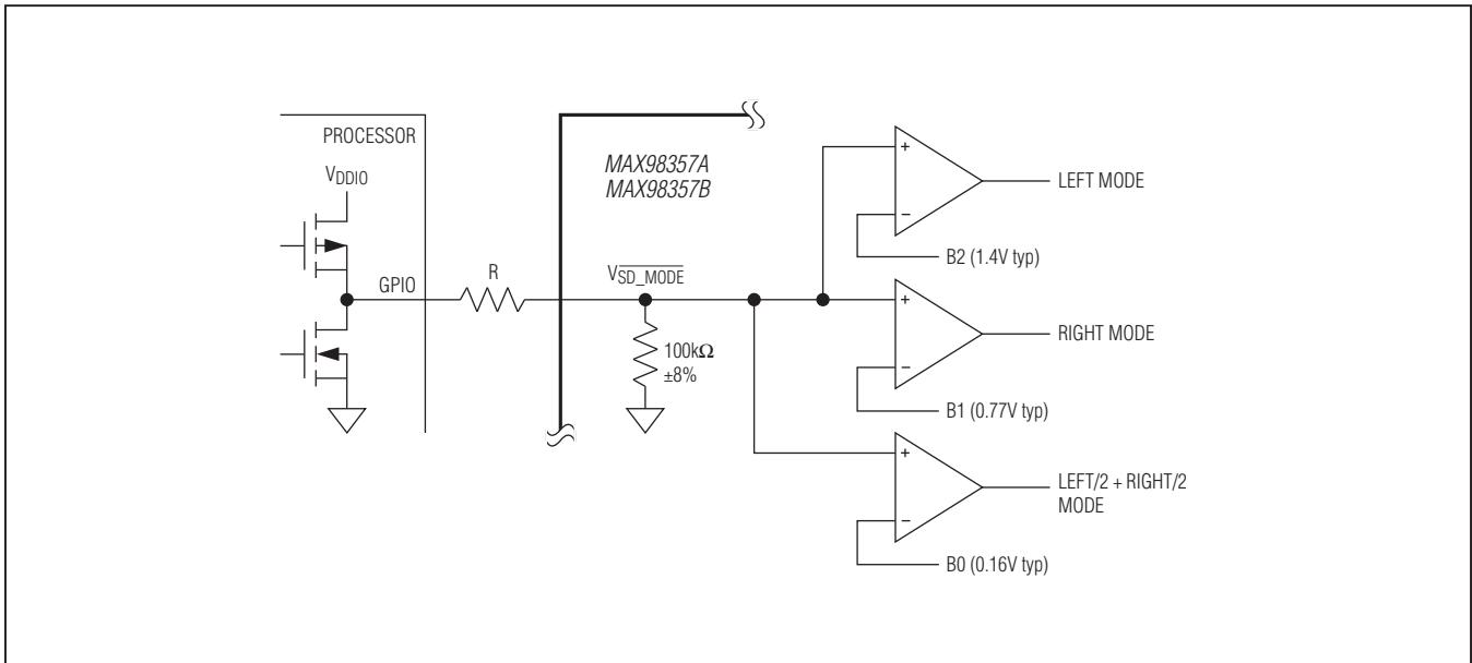
Figure 5. SD\_MODE Resistor Connected Using Push-Pull Driver
