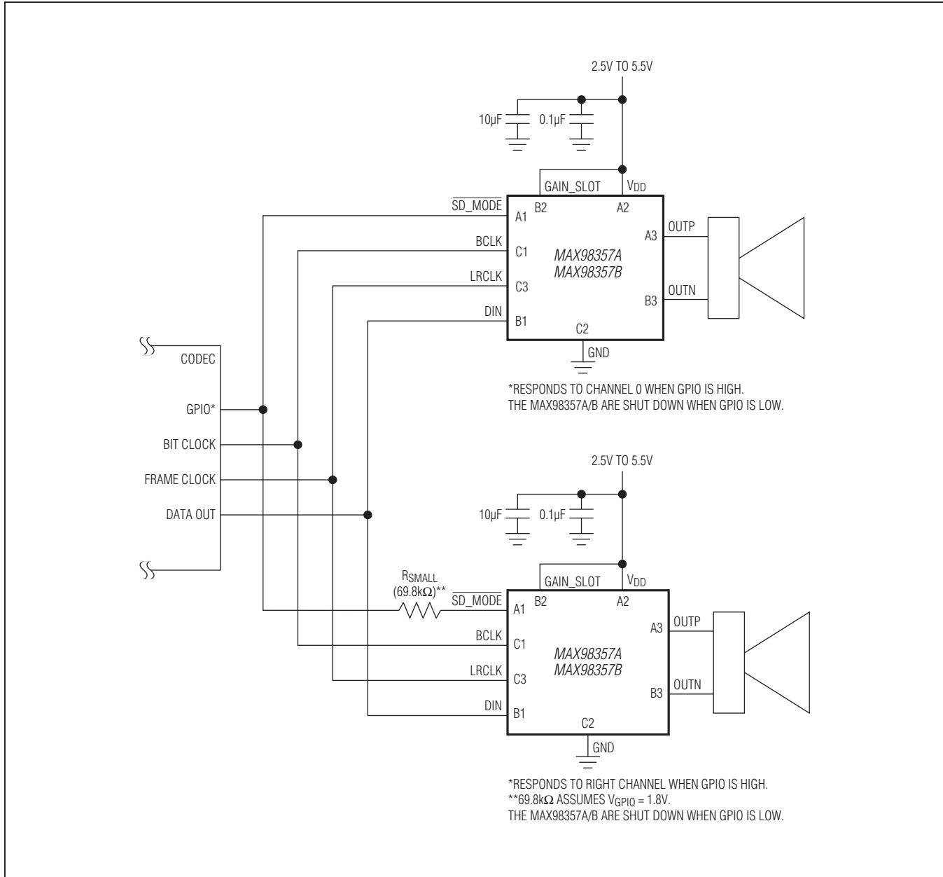
Figure 19. Stereo PCM Operation Using Two ICs
