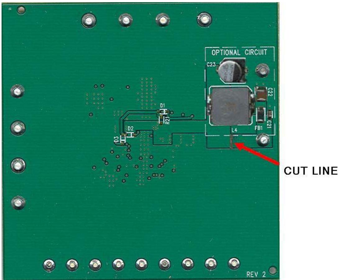
Figure 4. Cut Line for the EMI Filter Installation
