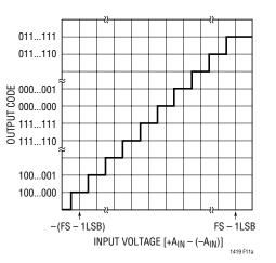
Figure 11a. LTC1419 Transfer Characteristics
