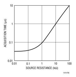
Figure 6. t<sub>ACQ</sub> vs Source Resistance
