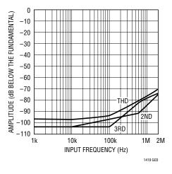
Figure 4. Distortion vs Input Frequency
