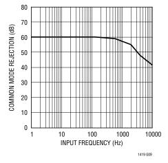
Figure 10a. CMRR vs Input Frequency
