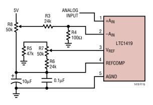
Figure 11b. Offset and Full-Scale Adjust Circuit
