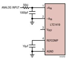
Figure 7. RC Input Filter
