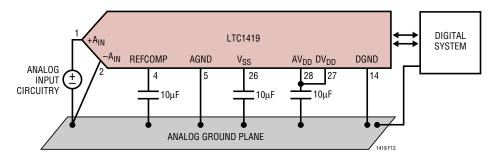
Figure 12. Power Supply Grounding Practice
