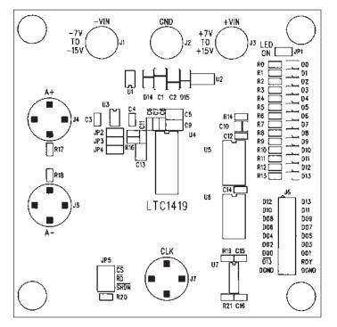
Figure 13b. Suggested Evaluation Circuit Board—Component Side Silkscreen
