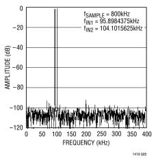
Figure 5. Intermodulation Distortion Plot
