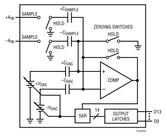
Figure 1. Simplified Block Diagram
