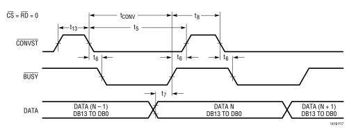
Figure 17. Mode 1b.  $\overrightarrow{\text{CONVST}}$  Starts a Conversion. Data Outputs Always Enabled ( $\overrightarrow{\text{CONVST}} = \_\_\_\_\_\_\_$ )
