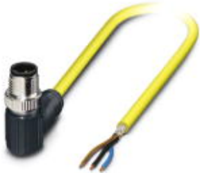
Sensor/Actuator cable, 3-position, PVC, Yellow RAL 1021, shielded, Plug angled M12-SPEEDCON, A-coded, on Free cable end, Cable length: 10 m
