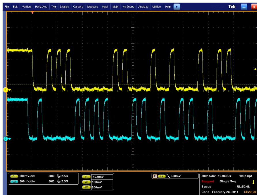
Figure 5. EMI4192 MIPI D-PHY LP Mode Measured Results
