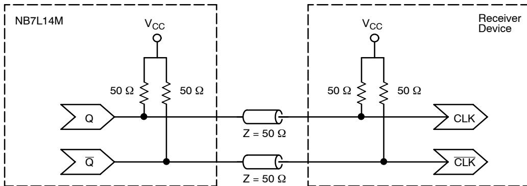
**Figure 9. Typical Termination for 16 mA Output Driver and Device Evaluation
