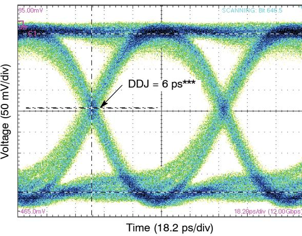
**Figure 7. Typical Output Waveform at 12 Gb/s with PRBS  $2^{23}-1$  ( $V_{inpp} = 75$  mV)**
