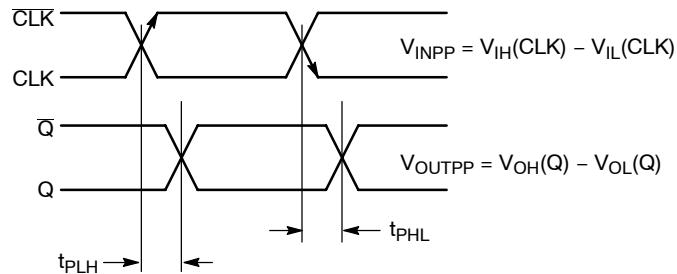
**Figure 8. AC Reference Measurement**
