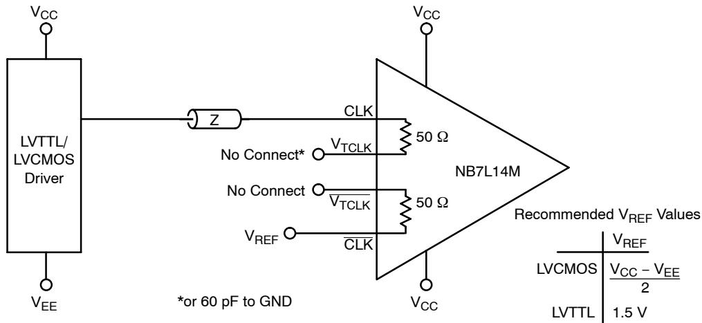
Figure 18. LVCMS/LVTTL to CML Receiver Interface
