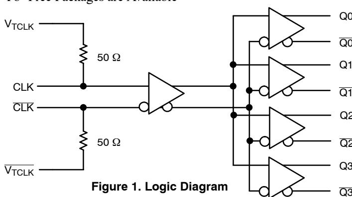
Figure 1. Logic Diagram
