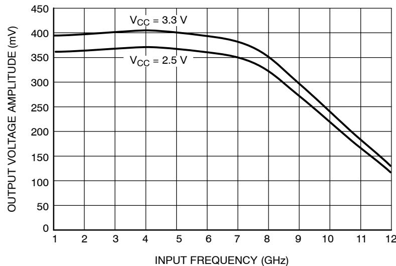
**Figure 3. Output Voltage Amplitude ( $V_{OUTPP}$ ) versus Input Clock Frequency ( $f_{in}$ ) at Ambient Temperature (Typical) ( $V_{INPP} = 400$  mV)**
