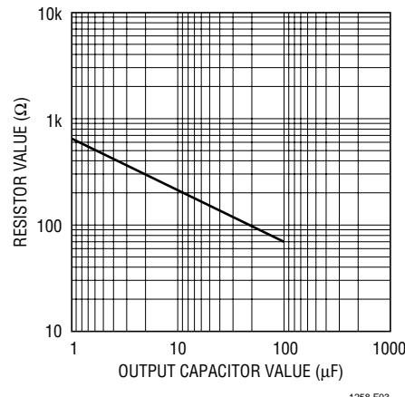
Figure 3. Damping Resistance vs Output Capacitor Value
