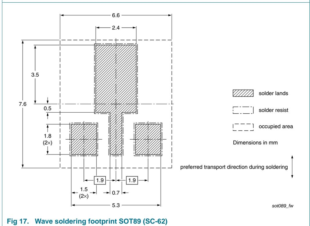
**Fig 17. Wave soldering footprint SOT89 (SC-62)**
