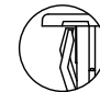
DETAIL VIEW VHP1, VHP3 & VHP5 HOLE PLUGS (No wing serrations for ease of removal)
