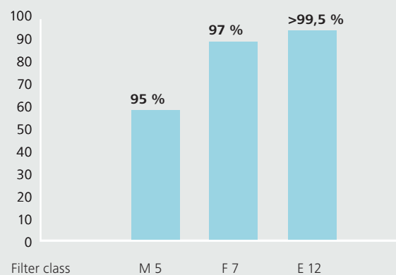
Medium filtration efficiency Em % against particle size 0,12 µm
