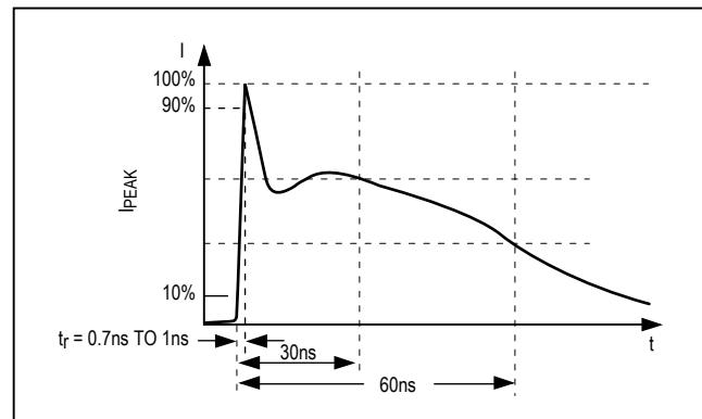
Figure 7. IEC 61000-4-2 ESD Generator Current Waveform
