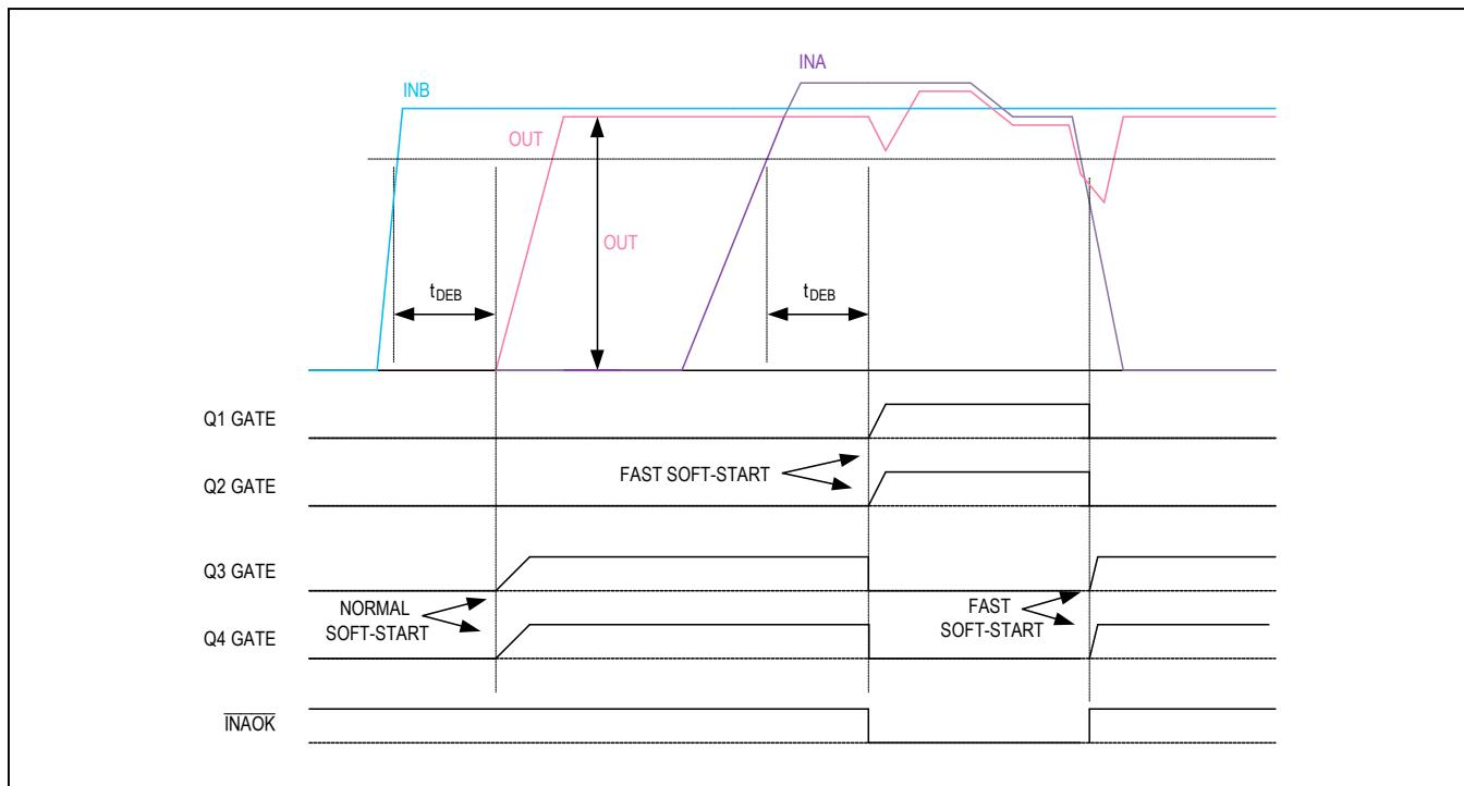
Figure 2. Automatic Switch Operation,  $PCON = 1$
