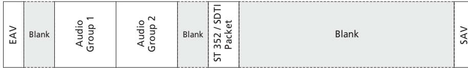
HANC with space between EAV and Ancillary Data (Audio Packets will be deleted)
