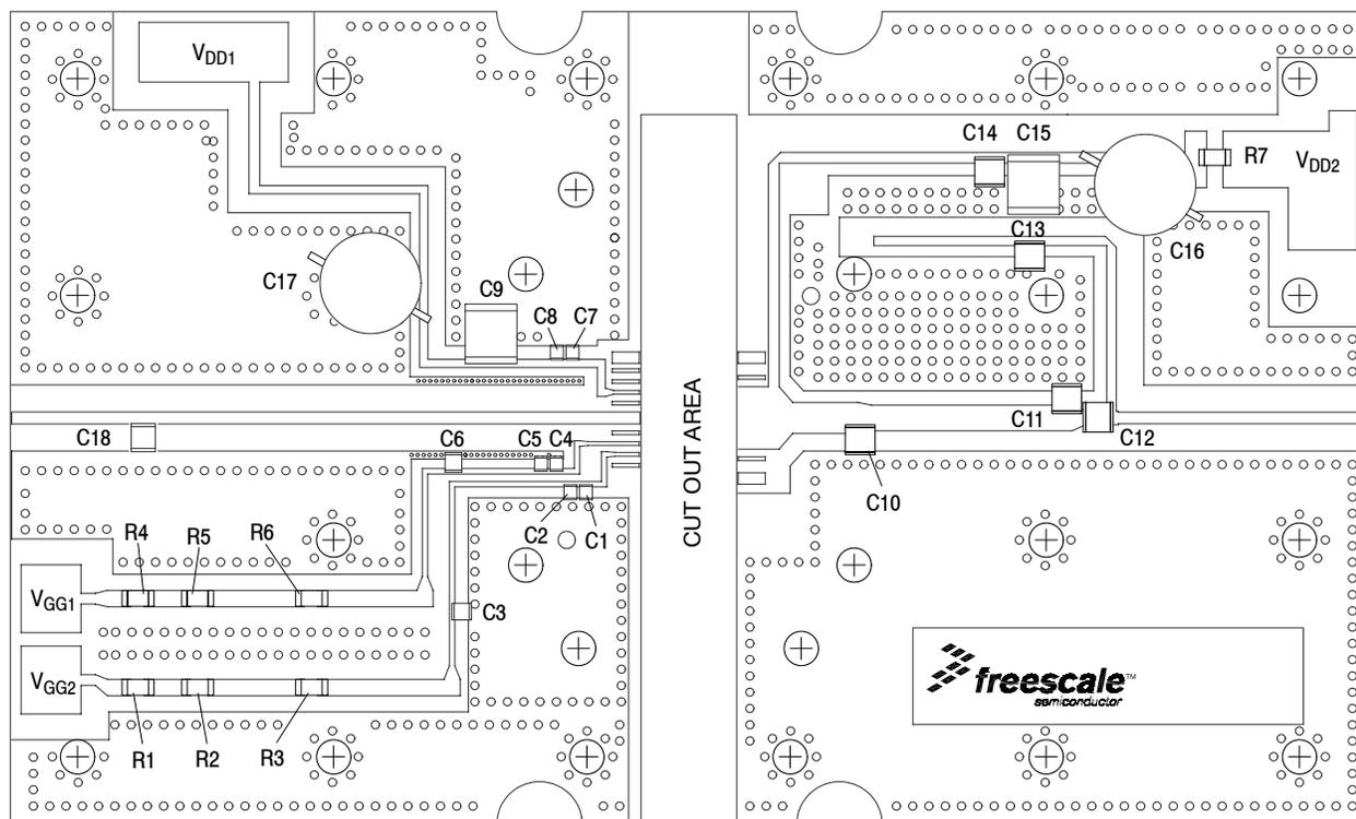
Figure 3. MMRF2005N Test Circuit Component Layout — 900 MHz
