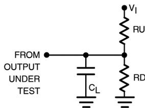
**Note:** Input driven by 50 Ω source terminated in 50 Ω, R<sub>U</sub> = R<sub>D</sub> = 500 Ω
