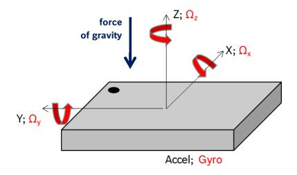
Figure 11: Orientation of sensing axis
