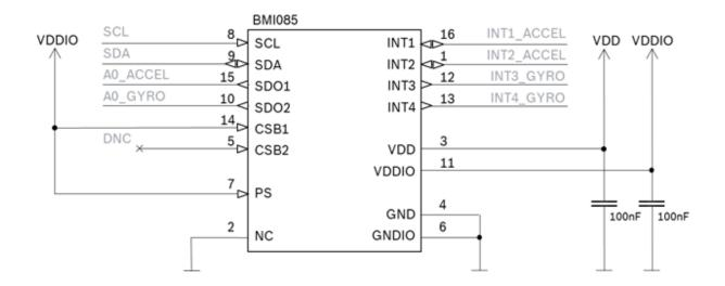
Figure 9: I<sup>2</sup>C connection
