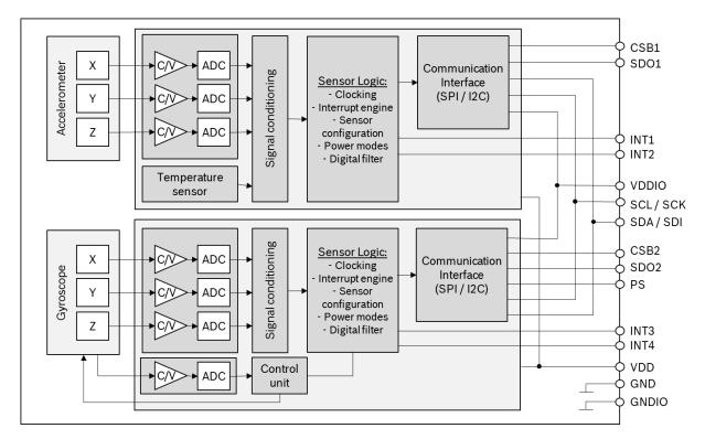
Figure 1: Block diagram of BMI085
