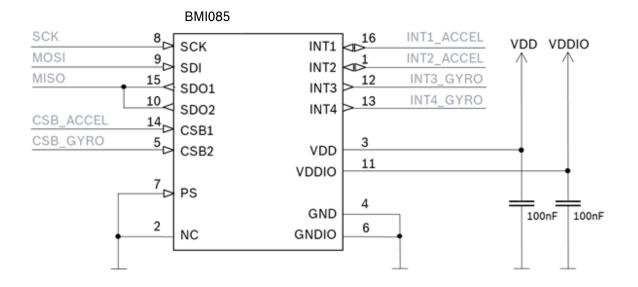
Figure 8: SPI connection
