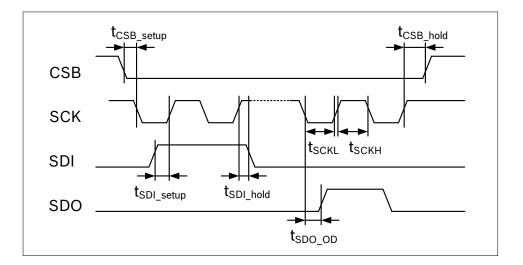
Figure 2: SPI timing diagram
