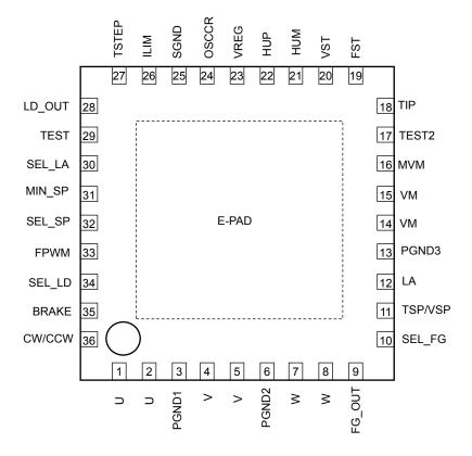
Note 1: Design the pattern in consideration of the heat design because the back side (E-PAD) has the role of heat radiation. The back side (E-PAD) should be connected to GND because it is connected to the back of the chip electrically.
