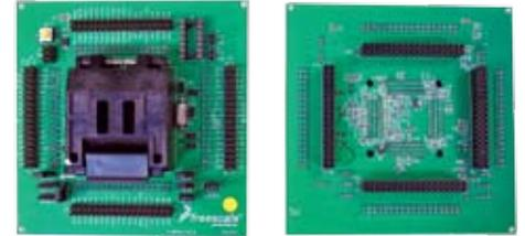
The cards include a CTI, Yamachi or Enflas zero insertion force (ZIF) socket, a background debug mode (BDM) connector and prototype connector ring. Configured for oscillator operation, the adaptor cards include support for a user supplied clock oscillator. They are compatible for use with any BDM tool.
