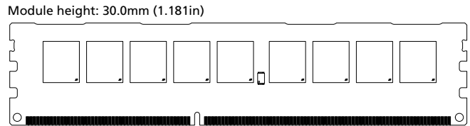
Figure 2: 240-Pin UDIMM (MO-269 R/C D1) PCBs 1483 & 1568
