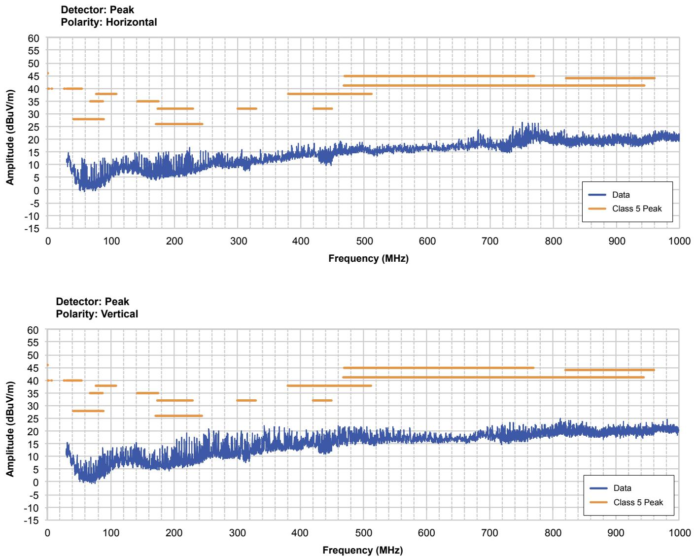
Figure 3. Radiated EMI Performance (Vertical/Horizontal),  $V_{IN} = 14V$ ,  $I_{OUT1,2,3} = 1A$
