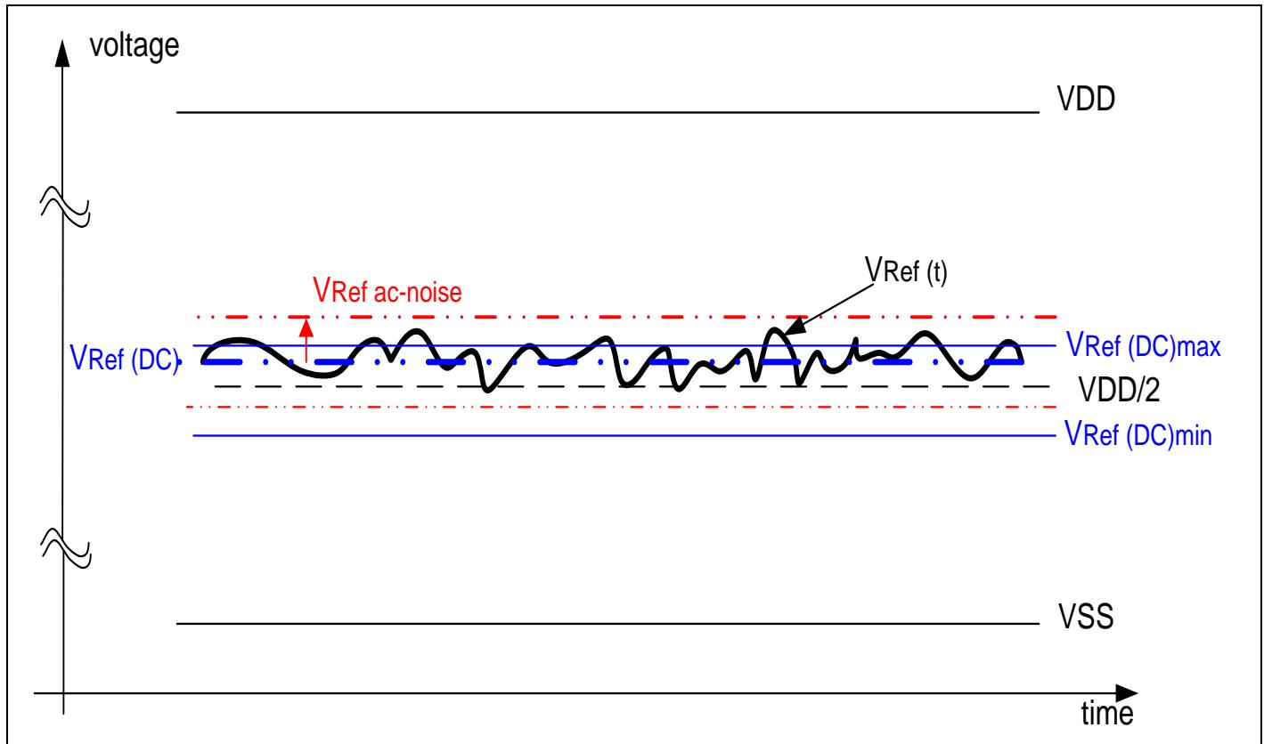
The voltage levels for setup and hold time measurements  $V_{IH(AC)}$ ,  $V_{IH(DC)}$ ,  $V_{IL(AC)}$  and  $V_{IL(DC)}$  are dependent on VRef.
