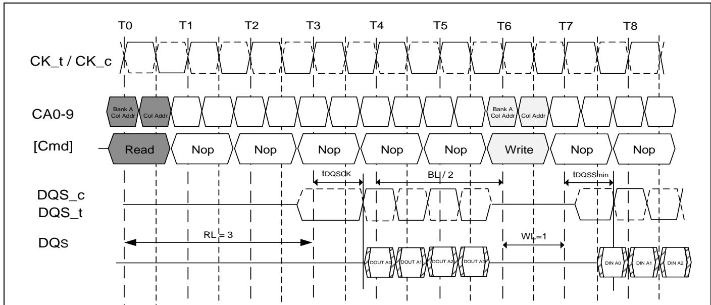
The minimum time from the burst read command to the burst write command is defined by the Read Latency (RL) and the Burst Length (BL). Minimum read to write latency is  $RL + RU(t_{DQSKmax}/t_{CK}) + BL/2 + 1 - WL$  clock cycles. Note that if a read burst is truncated with a Burst Terminate (BST) command, the effective burst length of the truncated read burst should be used as "BL" to calculate the minimum read to write delay.
