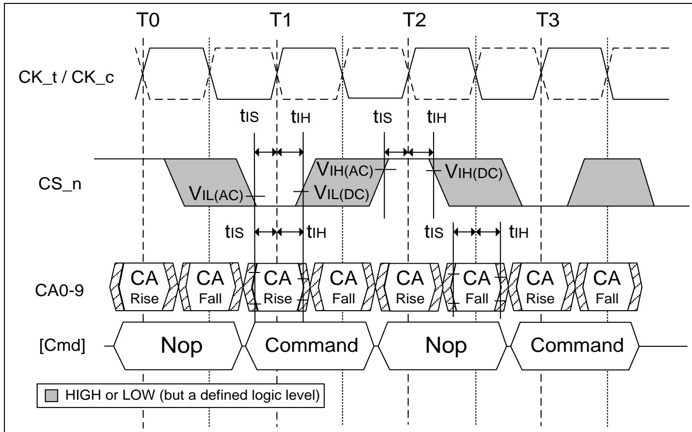
Note: Setup and hold conditions also apply to the CKE pin. See section related to power down for timing diagrams related to the CKE pin.
