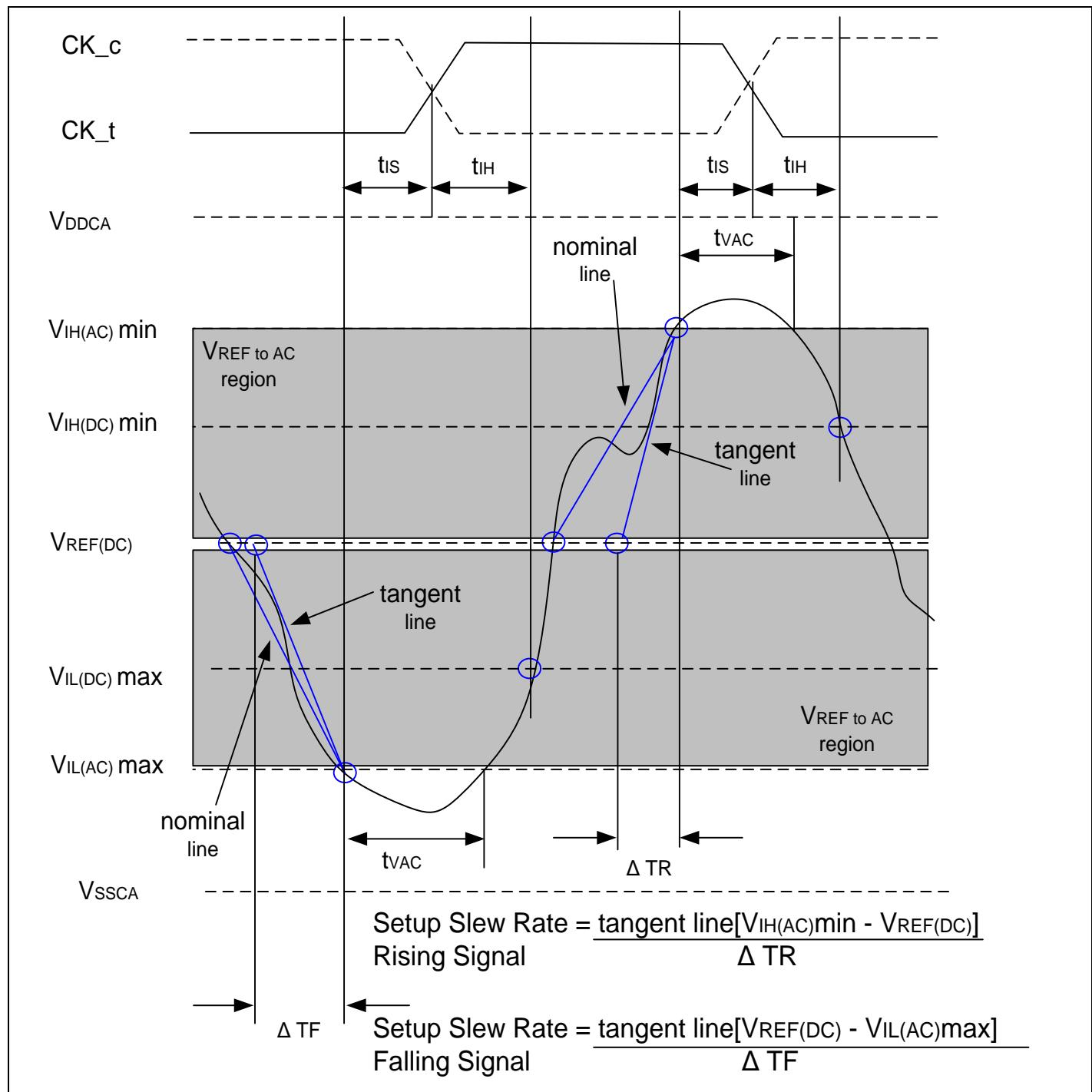
8.7.2.7 Tangent Line for Hold Time  $t_{IH}$  for CA and CS\_n with Respect to Clock
