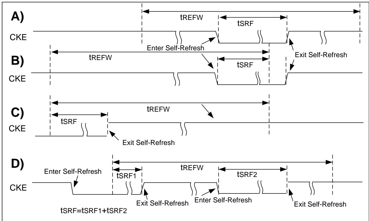
Several examples on how  $t_{SRF}$  is calculated:
