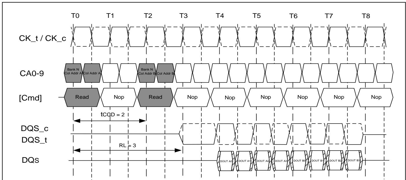
The seamless burst read operation is supported by enabling a read command at every other clock for BL = 4 operation, every 4 clocks for BL = 8 operation, and every 8 clocks for BL=16 operation.
