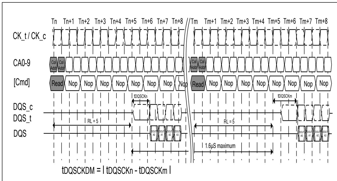
Note:  $t_{DQSCKDMmax}$  is defined as the maximum of  $\text{ABS}(t_{DQSCKn} - t_{DQSCKm})$  for any  $\{t_{DQSCKn}, t_{DQSCKm}\}$  pair within any  $1.6\mu\text{s}$  rolling window.
