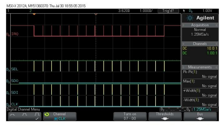
Above is the complete SPI & IRQ Timing diagram for #R<RSSI> <Packet > plus 12 byte data packet
