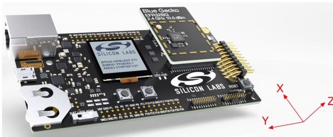
Figure 7.2. DUT: Radio Board with the Wireless Starter Kit Mainboard (Illustration)
