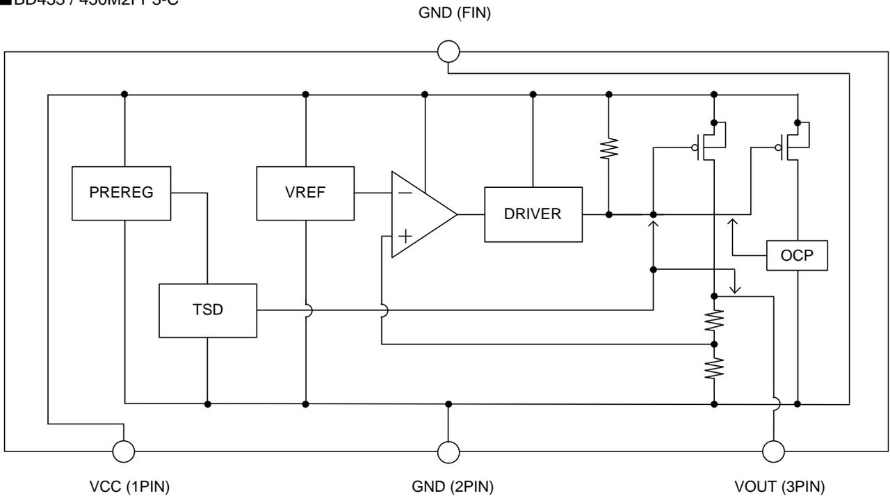
Figure 4. Block Diagrams
