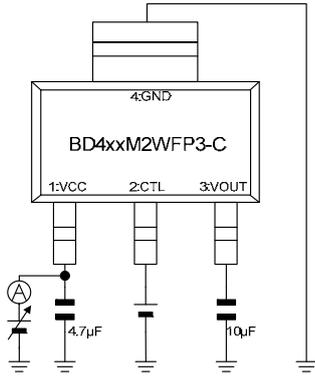
Measurement Setup for Figure 5, 7, 16, 17, 21, Figure 23, 25, 34, 35, 39
