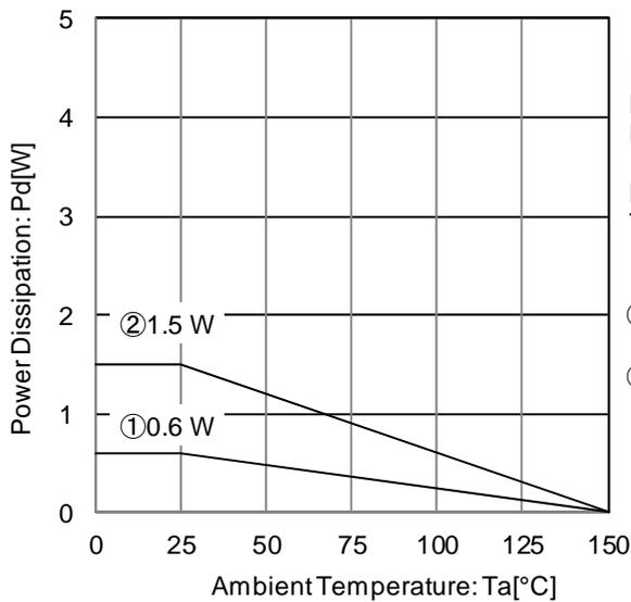
IC mounted on ROHM standard board based on JEDEC.
