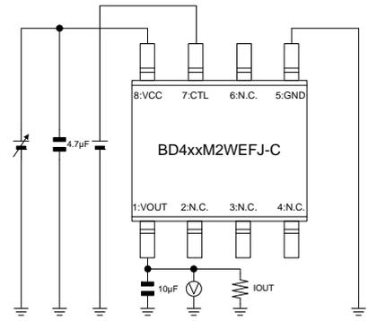
Measurement Setup for
