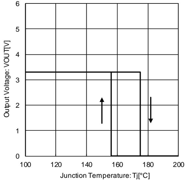
Figure 14. Output Voltage vs. Temperature (Thermal Shut Down)
