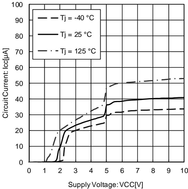
Figure 25. Circuit Current vs. Power Supply Voltage
