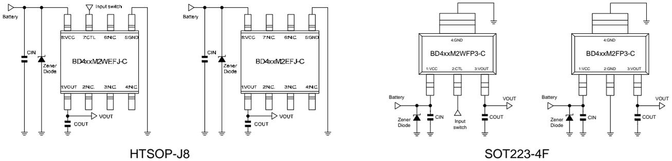
Figure 46. Sample Application Circuit 1
