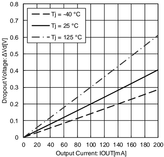
Figure 11. Dropout Voltage ( $V_{CC} = 3.135\text{ V}$ )
