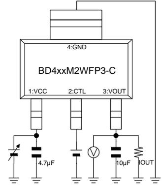
Measurement Setup for Figure 9, 27
