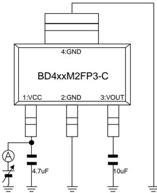
Measurement Setup for
