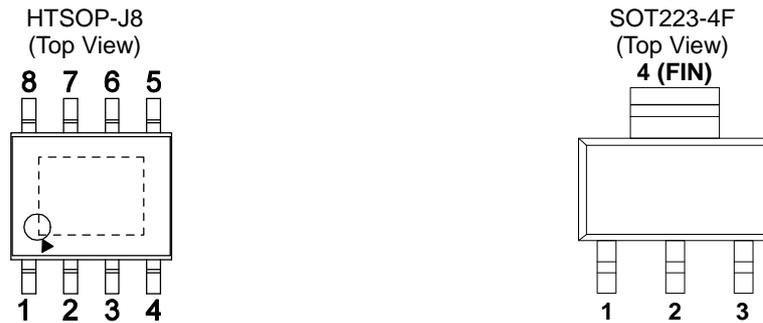
Figure 3. Pin Configuration
