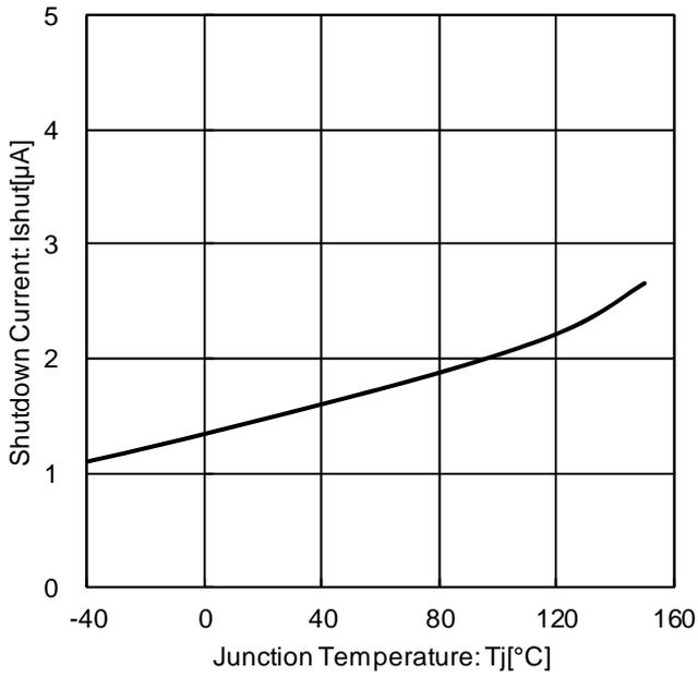
Figure 39. Shut Down Current vs. Temperature (CTL = 0 V)
