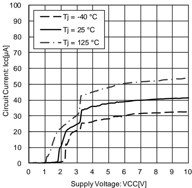
Figure 7. Circuit Current vs. Power Supply Voltage
