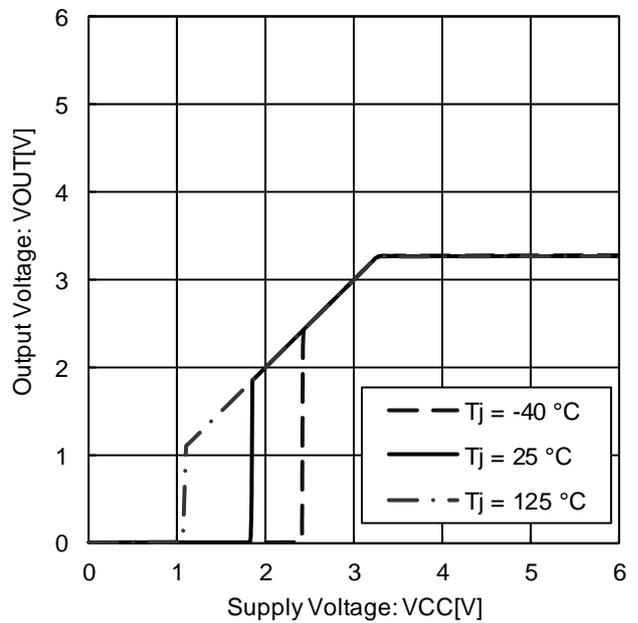
Figure 8. Output Voltage vs. Power Supply Voltage ( $I_{OUT} = 0\text{ mA}$ )
