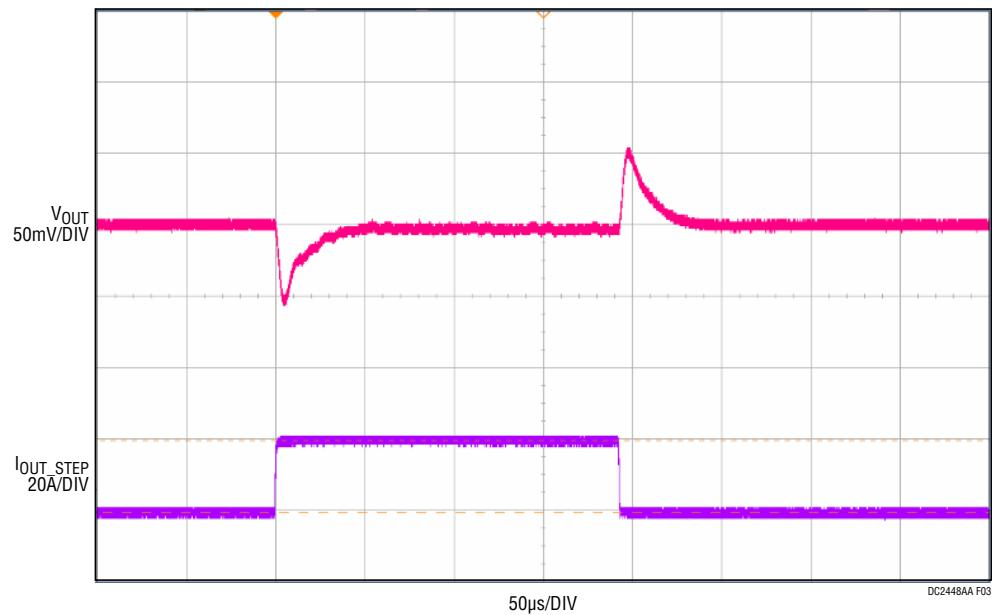
Figure 3. Measured Load Transient
