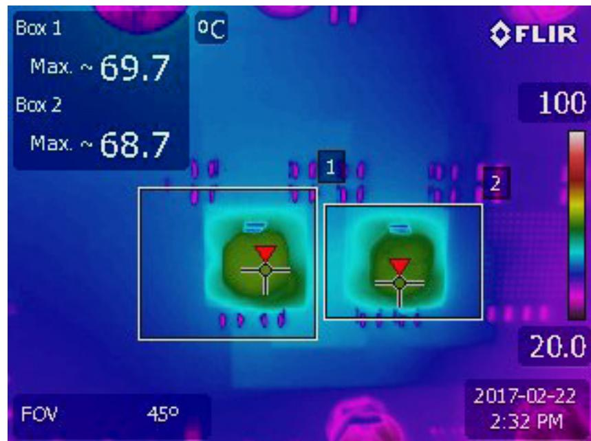
Figure 4. Thermal Capture at  $V_{IN} = 12V$ ,  $V_{OUT} = 0.9V$ , 80A ( $T_A = 25^{\circ}\text{C}$ , 200LFM Airflow and No Heat Sink)
