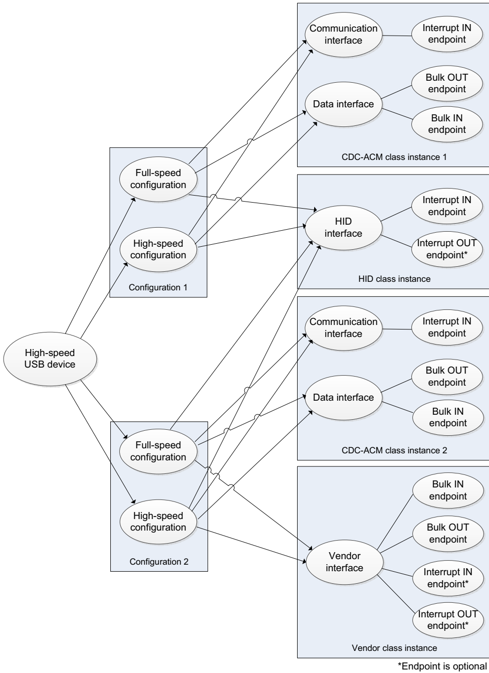
Figure 5-2 Complex Composite High-Speed USB Device Structure
