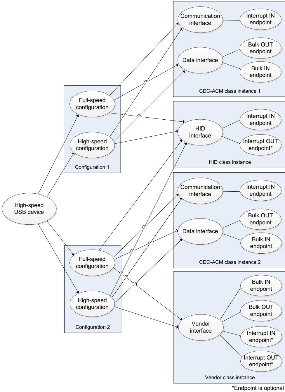
Figure 5-2 Complex Composite High-Speed USB Device Structure
