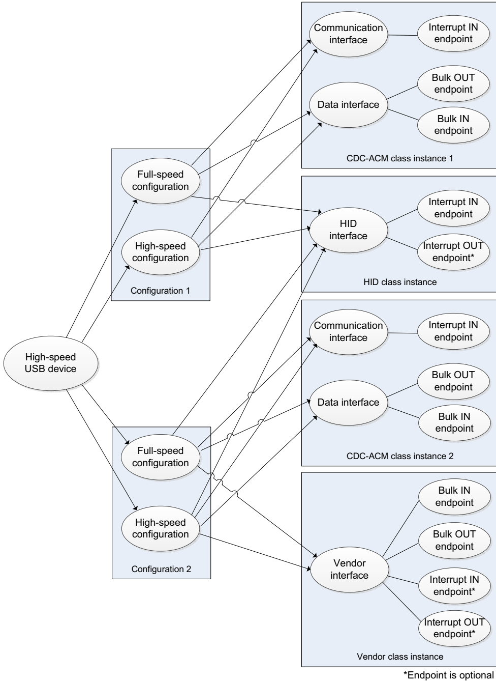
Figure 5-2 Complex Composite High-Speed USB Device Structure
