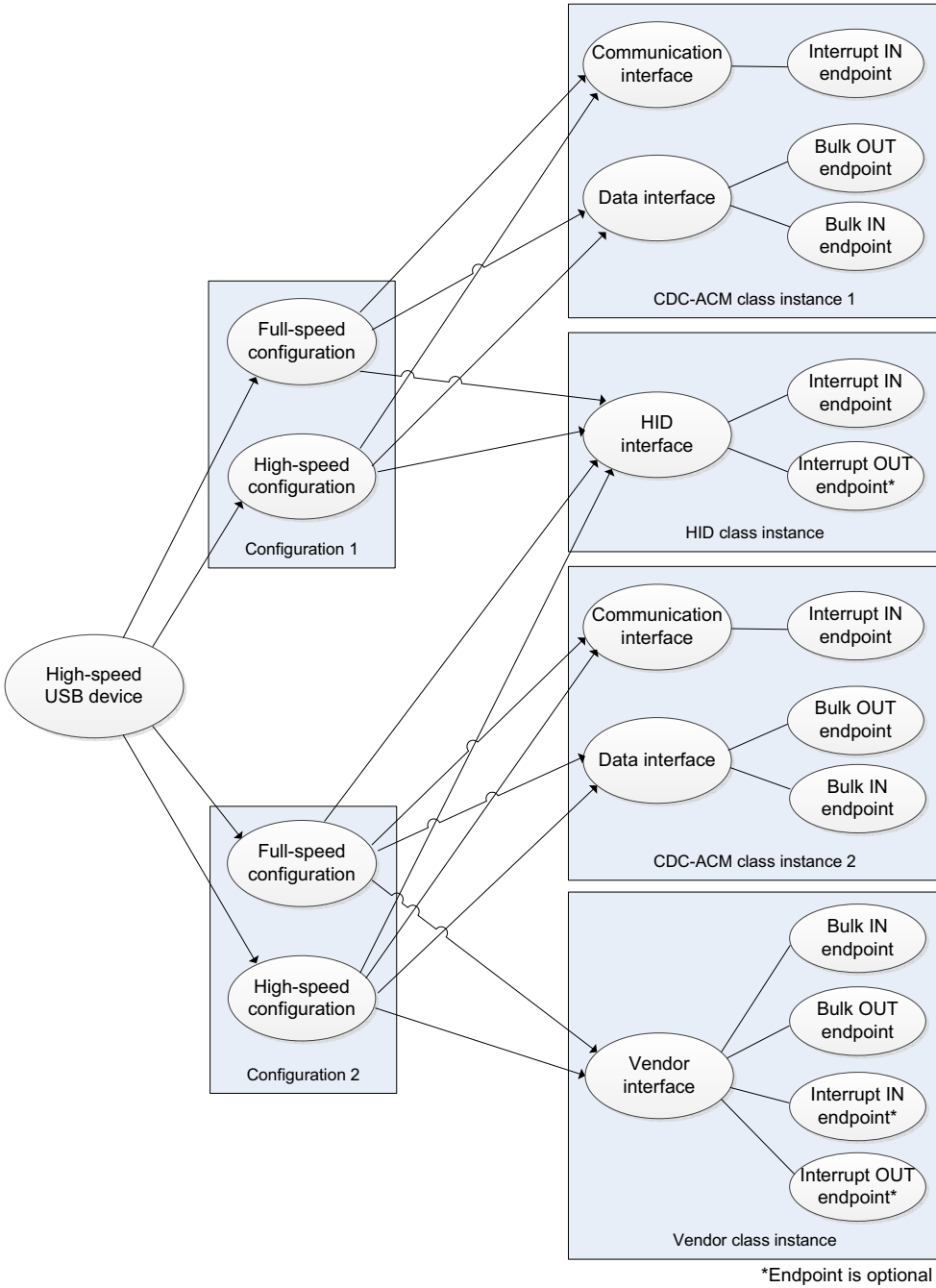
Figure 5-2 Complex Composite High-Speed USB Device Structure
