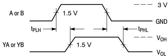
**Figure 3. Switching Waveform**
