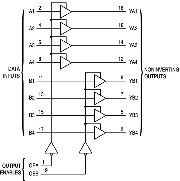
**Figure 1. Logic Diagram**
