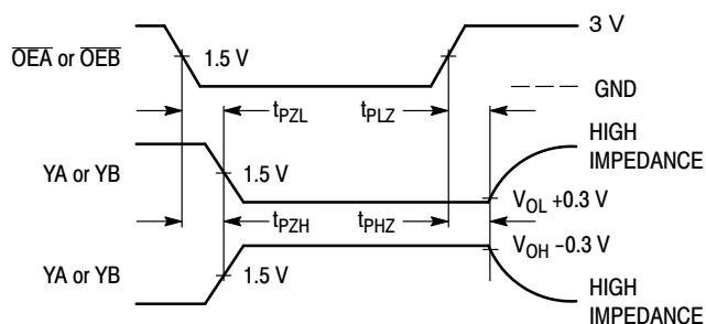
**Figure 4. Switching Waveform**
