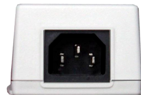
Power Supply Inserter AC Power IN (90-264VAC)@120V/230
