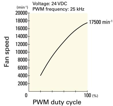
**9WL0424P3G001** With pulse sensor with PWM control function
