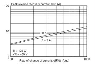
Fig.8. Typical peak reverse recovery current, I<sub>rrm</sub> as a function of rate of change of current dI<sub>r</sub>/dt.
