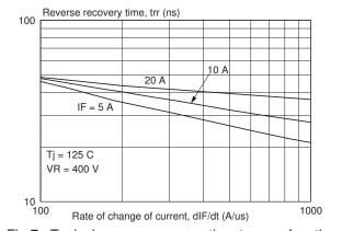
Fig.7. Typical reverse recovery time  $t_{rr}$ , as a function of rate of change of current  $dl_{r}/dt$ .
