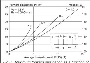
Fig.3. Maximum forward dissipation as a function of average forward current; rectangular current waveform where  $I_{F(AV)} = I_{F(RMS)} \times \sqrt{D}$ .
