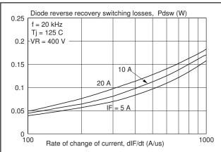
Fig.4. Typical reverse recovery switching losses in diode, as a function of rate of change of current dl<sub>F</sub>/dt.
