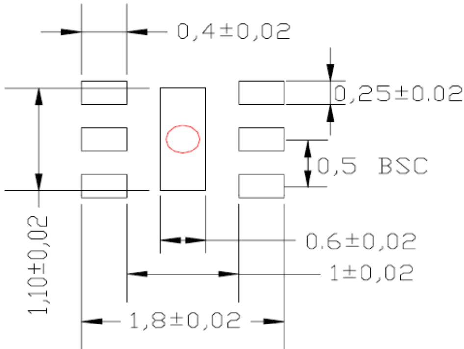
**Red circle** indicates Thermal Via. Size should be .300-.350 mm in diameter and it should be connected to GND plane for maximum thermal performance.
