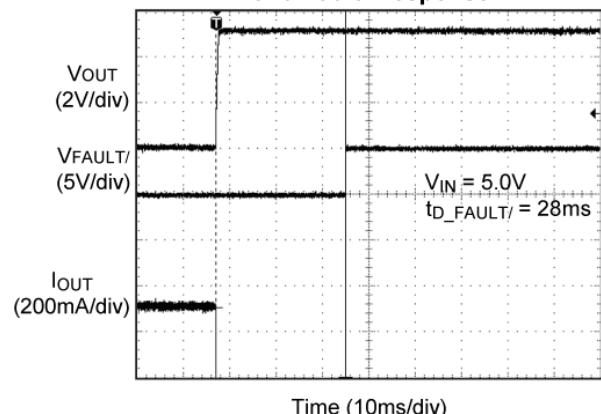
**2098 Output Recovery from Short Circuit and FAULT/Response**
