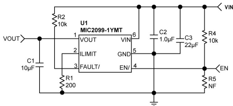
**Figure 9. MIC2099-1 Schematic**
