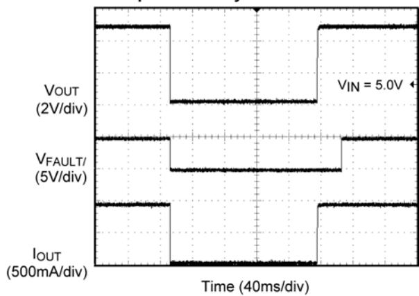
**2099 Output Recovery from Thermal Shutdown**
