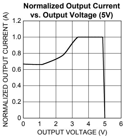
Figure 3. Normalized Output Current vs. Output Voltage
