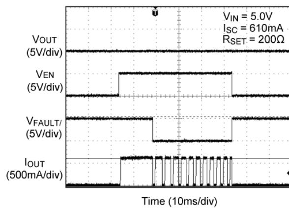
**2097 Enabled into an Overcurrent Condition**
