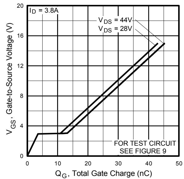
**Fig 6.** Typical Gate Charge vs.
