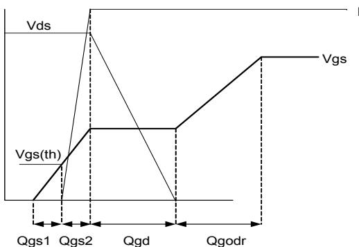
**Fig 9a.** Basic Gate Charge Waveform
