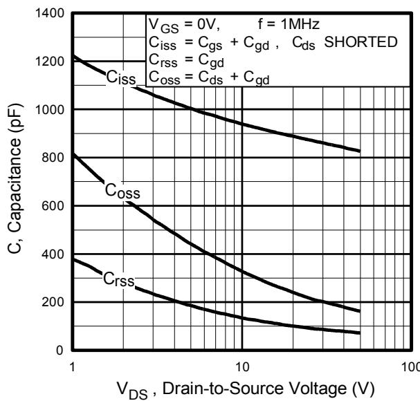
**Fig 5.** Typical Capacitance vs.
