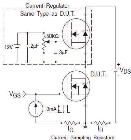
**Fig 9b.** Gate Charge Test Circuit
