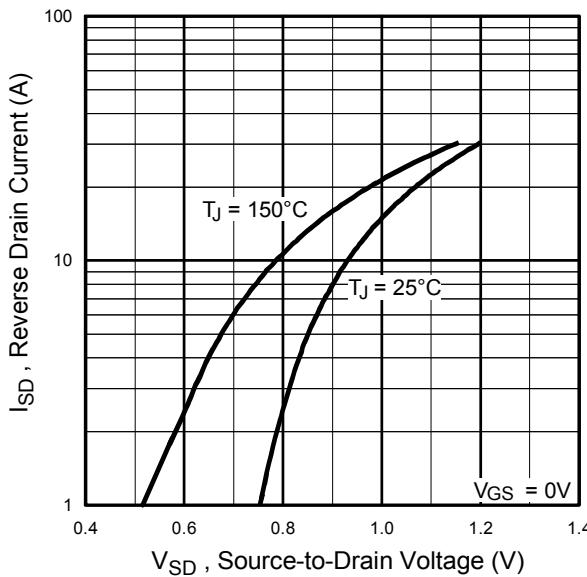
**Fig. 7** Typical Source-to-Drain Diode
