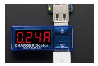
If you want to check the exact current draw during charge, try out a Charger Doctor between the USB port and charger. (https://adafru.it/dvm)
