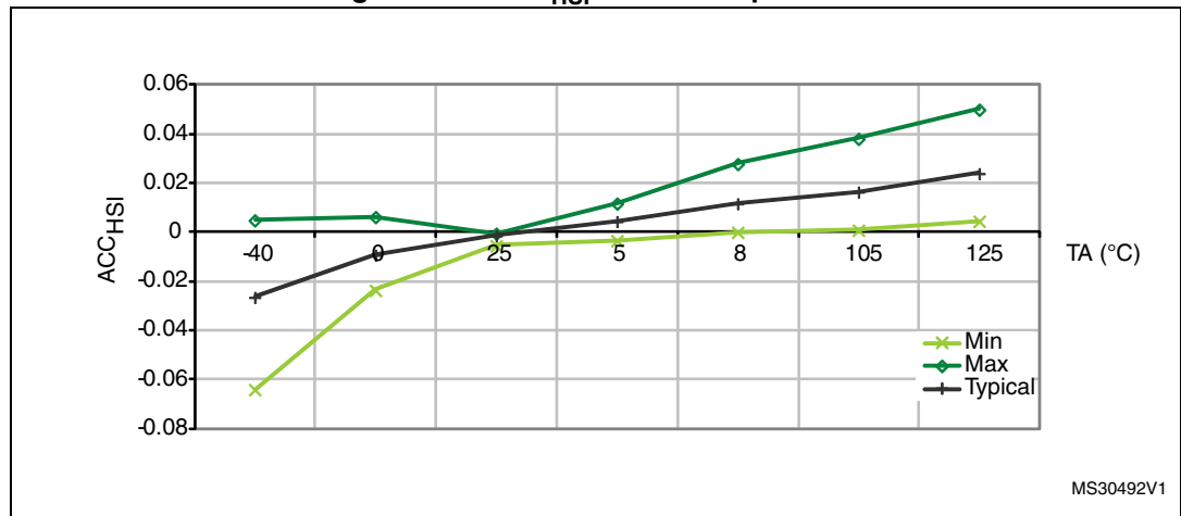
Figure 27. LACC_{HSI} versus temperature
