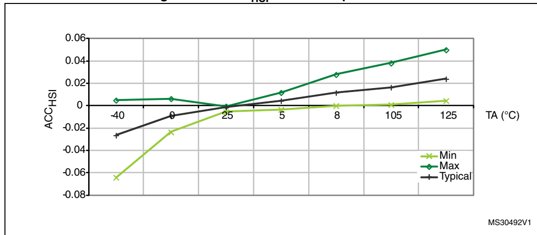
Figure 27. LACC_{HSI} versus temperature
