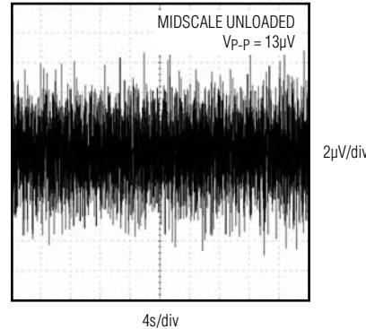
**0.1Hz TO 10Hz OUTPUT NOISE, INTERNAL
