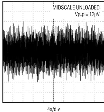
**0.1Hz TO 10Hz OUTPUT NOISE, INTERNAL
