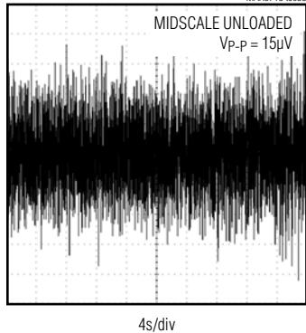
**0.1Hz TO 10Hz OUTPUT NOISE, INTERNAL
