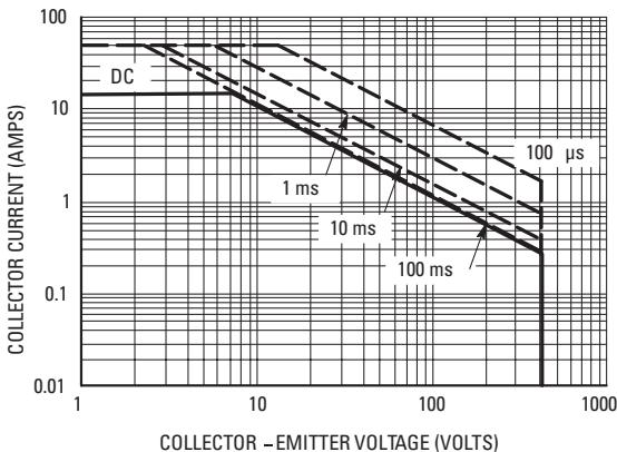
**Figure 16. Single Pulse Safe Operating Area**
