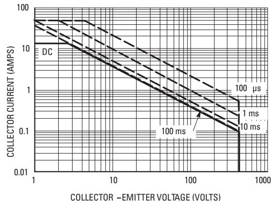
**Figure 17. Pulse Train Safe Operating Area**
