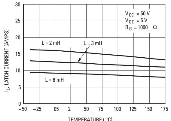
**Figure 11. Typical Open Secondary Latch Current vs Temperature**
