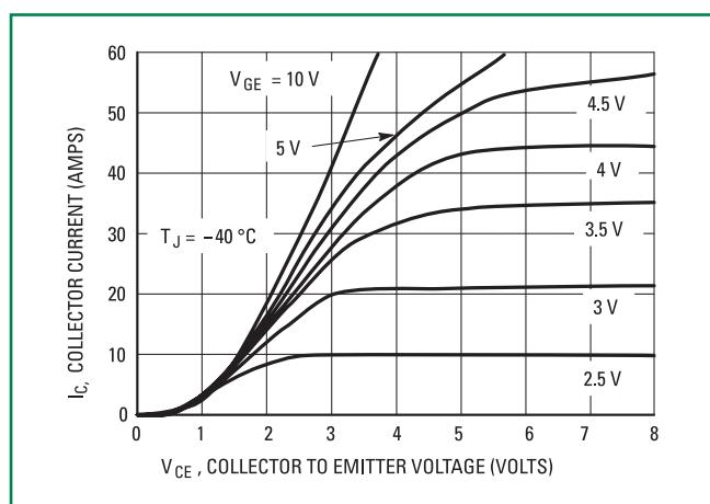
**Figure 3. Output Characteristics**
