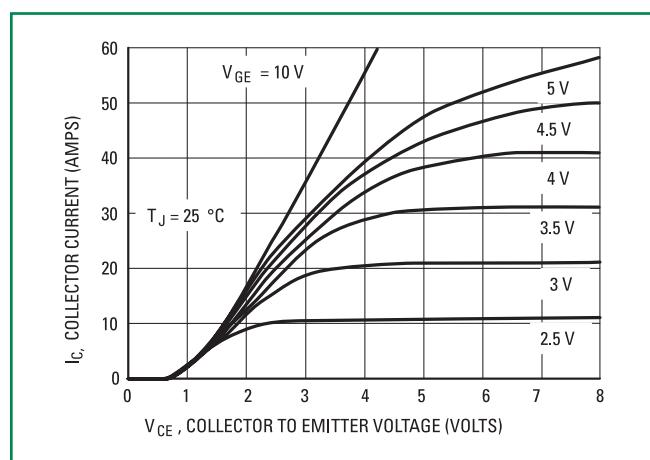
**Figure 2. Output Characteristics**
