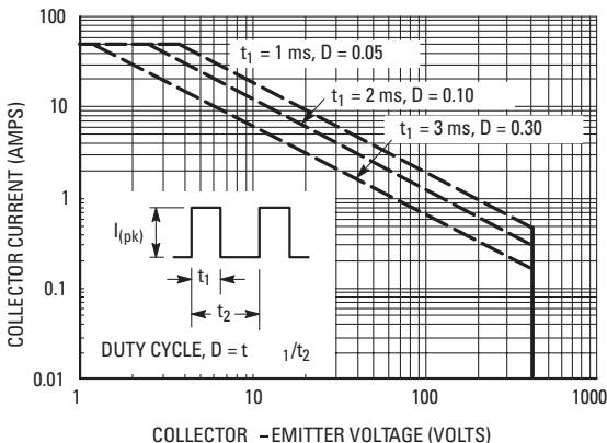
**Figure 18. Pulse Train Safe Operating Area**
