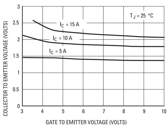
**Figure 7. Collector-to-Emitter Voltage vs Gate-to-Emitter Voltage**
