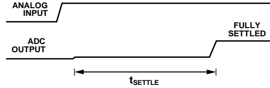
Figure 61. Step Input with Single Cycle Settling
