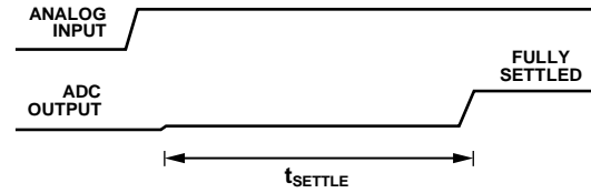
Figure 61. Step Input with Single Cycle Settling
