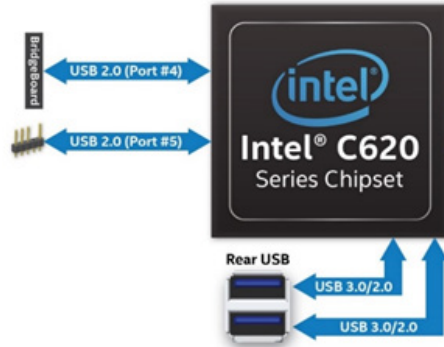
Figure 70. USB Ports Block Diagram
