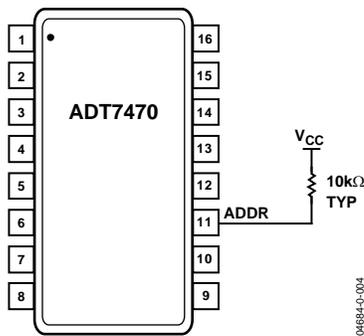
Figure 4. SMBus Address = 0x5E or 0x2F (Pin 11 = 1)
