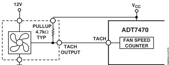
Figure 20. Fan with Tach Pull-Up to  $V_{CC}$
