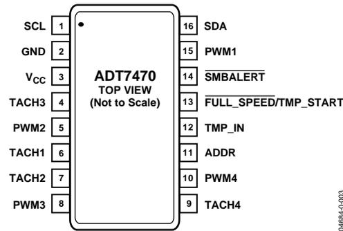
Figure 3. Pin Configuration
