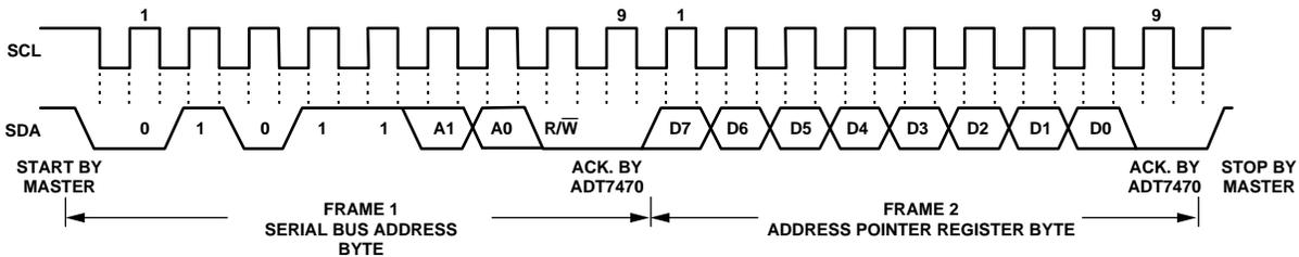
Figure 8. Writing to the Address Pointer Register Only
