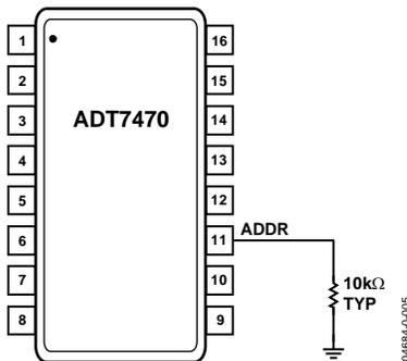
Figure 5. SMBus Address = 0x58 or 0x2C (Pin 11 = 0)
