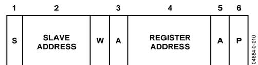
Figure 10. Setting a Register Address for Subsequent Read
