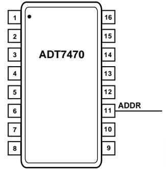
Figure 6. SMBus Address = 0x5C or 0x2E (Pin 11 = Floating)
