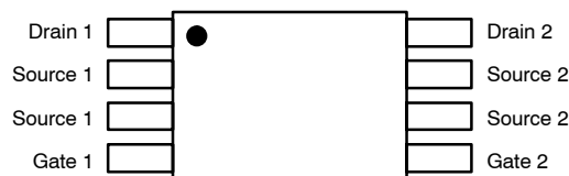
Figure 3. Pinouts for Dual-Die TSSOP
