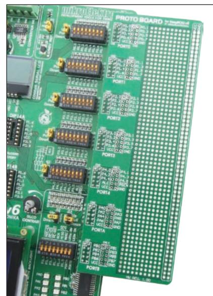
Figure 1-4: Proto board connected to Easy8051 v6
