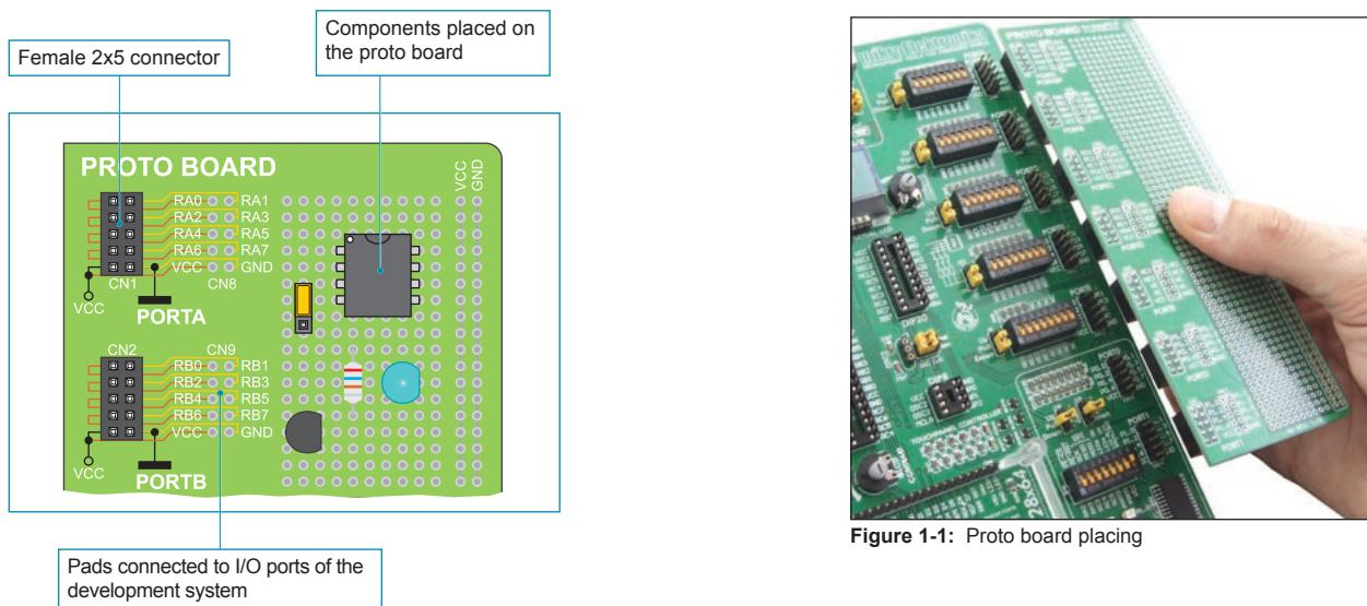
Figure 1-1: Proto board placing
