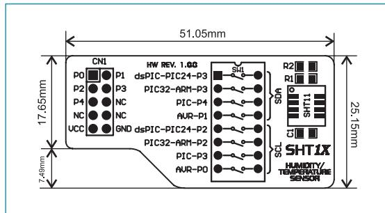
Figure 3: Dimensions of the SHT1X additional board
