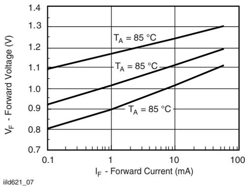
Fig. 7 - Forward Voltage vs. Forward Current
