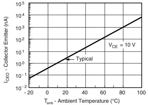
Fig. 9 - Collector Emitter Leakage vs. Temperature
