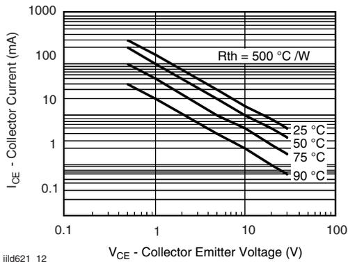
Fig. 12 - Maximum Collector Current vs. Collector Voltage
