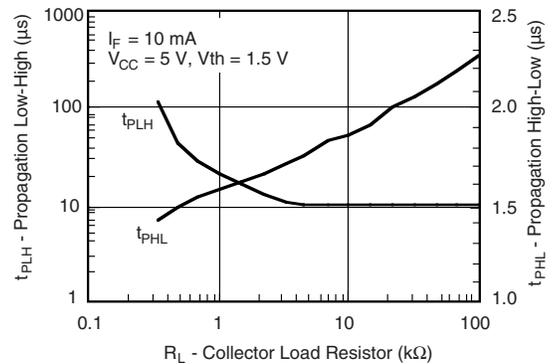
Fig. 10 - Propagation Delay vs. Collector Load Resistor
